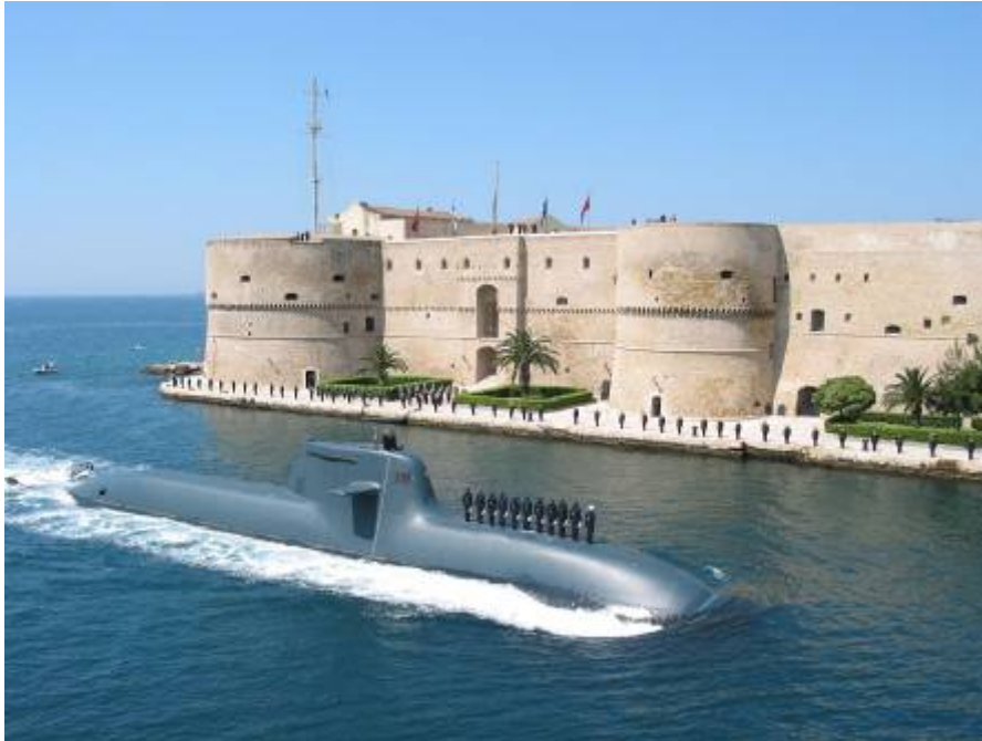
U212A type submarine of the Italian navy equipped with fuel cell technology from Siemens near Taranto, Italy.
