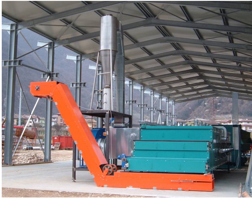
Sludge Belt Dryer from Siemens Water Technologies.
